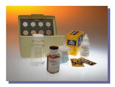
The Hydrogen Sulfide Detection Kit provides a rapid and inexpensive (qualitative) procedure for detecting the presence of  $H_2S$ . This colorimetric method uses the same Hydrogen Sulfide Test paper discs as the Garrett Gas Train and can detect as little as 0.3 ppm  $H_2S$ .
